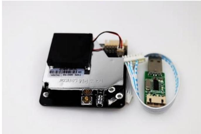
Nova PM sensor SDS011 High precision laser pm2.5 air quality detection sensor module Super dust dust sensors, digital output
